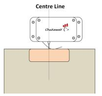
Once satisfied that the positioning is correct, use 4 of the large screws provided to screw the Motor Assembly in place. If mounted in exposed environment, apply sealant along the upper rear edge of the assembly. <u>With the door closed</u>, tie the cord to the door ensuring that there is about one to two inches of slack in the cord. It is very important that there is slack in the cord! (Either tie a large knot at the base of the hole or tie the cord back on itself just above the hole).
