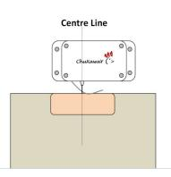
Use the 4 screws provided to screw the Motor Assembly in place. If mounted in exposed environment, apply sealant along the upper rear edge of the assembly. With the door closed, tie the cord to the door ensuring that there is about one inch of slack in the cord. Either tie a large knot at the base of the hole or tie the cord back on itself just above the hole.
